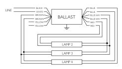
Diag. 9 Note: Insulate unused leads individually as shown on a ballast label
