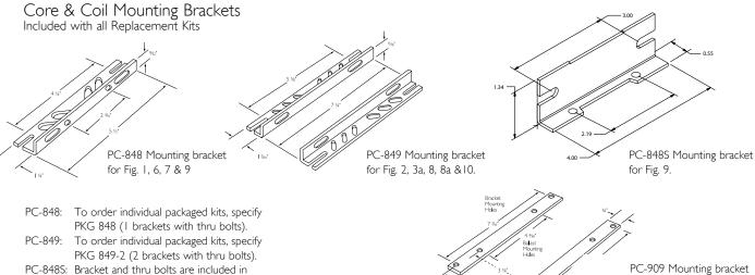
PC-909 Mounting bracket for Fig. 2, 3a & 8 when used with power-door roadway fixtures
