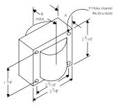
Fig. 9 (2<sup>5</sup>/<sub>8</sub>'' × 2<sup>3</sup>/<sub>16</sub>'' Reactor Core)
