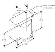
Fig. 9 (2<sup>5</sup>/<sub>8</sub>'' × 2<sup>3</sup>/<sub>16</sub>'' Reactor Core)
