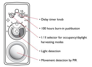
The sensor will automatically lengthen the delay time when the sensor detects presence directly after the moment it has given the signal "no presence" (will double the delay time once). Reduce the frustration of false "no presence" triggers with the smart timer function.
