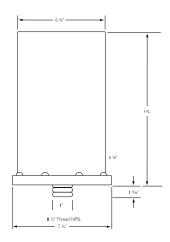
All weatherproof high pressure sodium lamp ballasts are furnished with an Philips Advance long range ignitor built into the ballast enclosure. Maximum lamp-to-ballast distance is 50 ft. (except 1000W ballasts which are 75 ft.)
