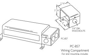
Wiring Compartment For end mounting, includes (5) 7/8" dia. knockouts. May be used with or without PC-625 Mtg. Brkt. Kit
