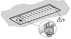
LuxSense mounted with a lamp clip (For use with T5 lamps only). Not for use with T5/HO lamps.
