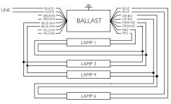
Diag, 14 Note: Insulate unused leads individually as shown on a ballast label
