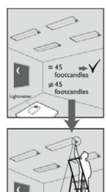
Measure the light level under each ActiLume 1-10V sensor with no or negligible daylight contribution.
