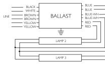
Diag, 5 Note: Insulate unused leads individually as shown on a ballast label
