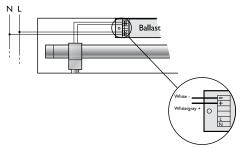
Connecting diagram of the sensor to the ballast
