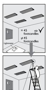
igntmeter readin of 45 footcandles Measure the light level under each LuxSense sensor with no or negligible daylight contribution.
