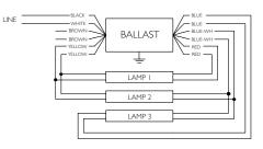
Diag, 8 Note: Insulate unused leads individually as shown on a ballast label
